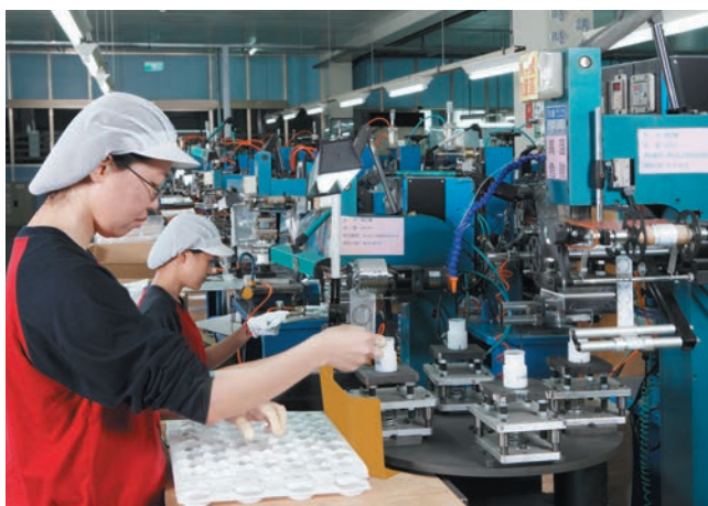
燙金課 (半自動燙金) Hot Stamping Sec. (Semi-automatic Hot Stamping Machine)
